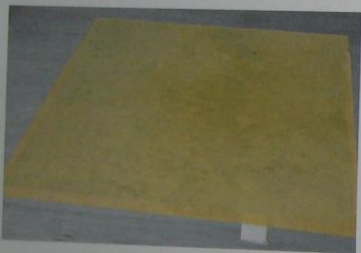
7. Turn the wet composite over onto the surface of a board for drying. Use a clean, dry, wide brush (or the dry brush you previously used) to smooth out any air pockets and ensure good contact at the margins of the wet assembly.
